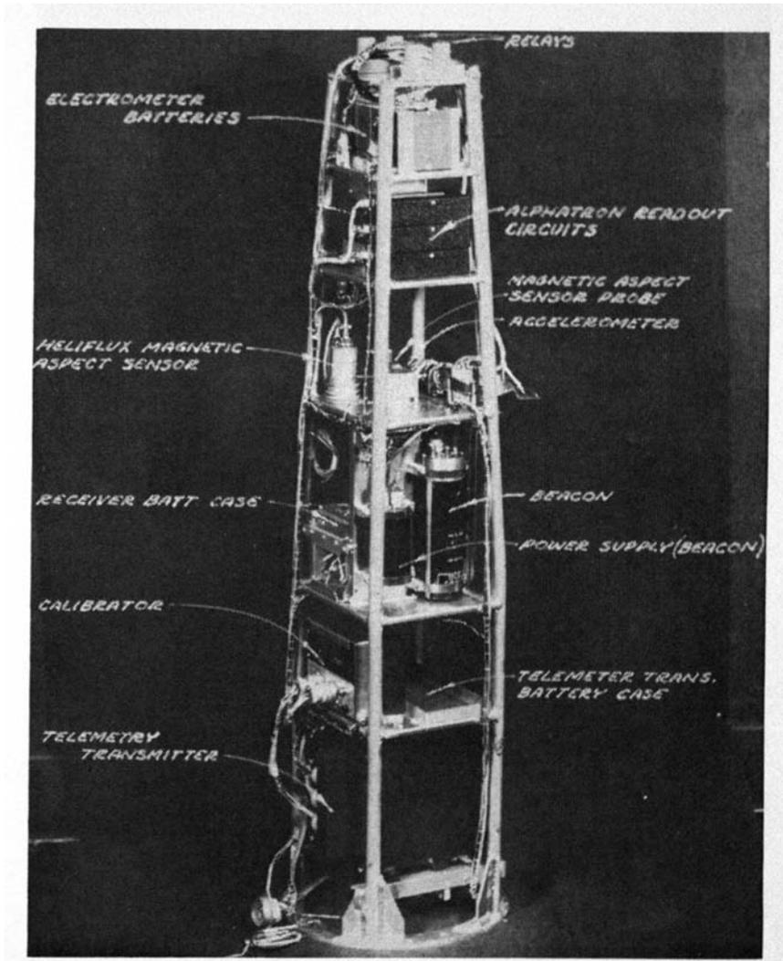
Figure 1. Aerobee Payload Assembly
