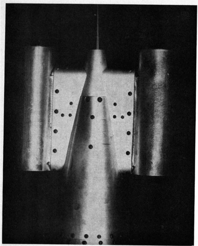
Figure 2. Aerobee Nose Tip With Gerdien Condensers
