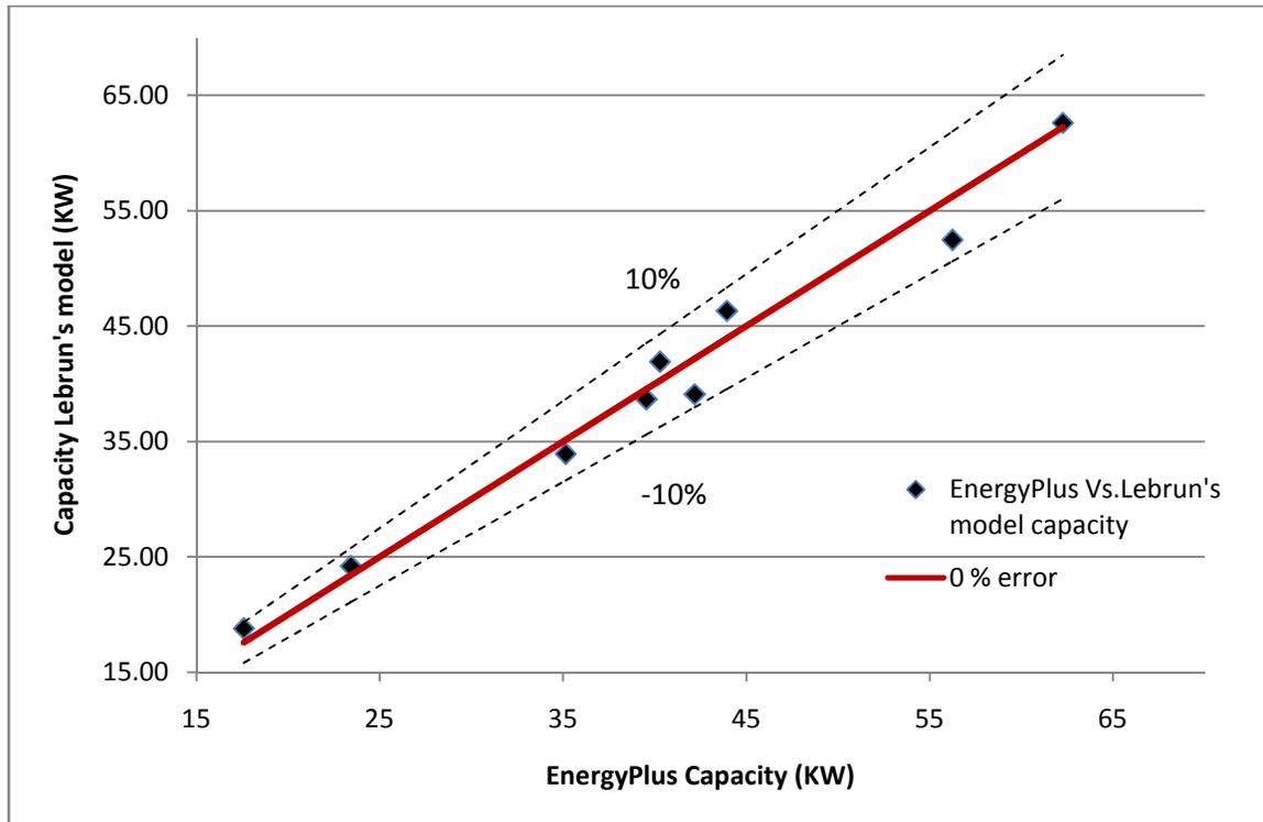
Fig. 5.3 EnergyPlus Vs Lebrun model capacity (KW)
