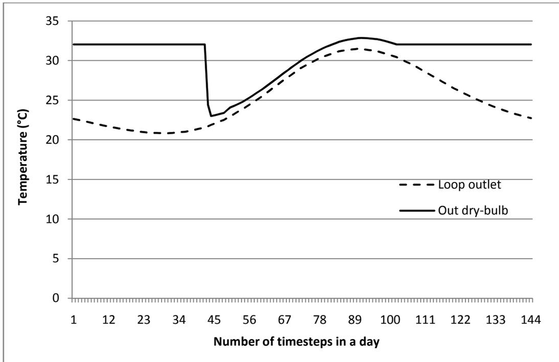
Fig 6.9 Air dry-bulb and loop outlet temperature on the design day
