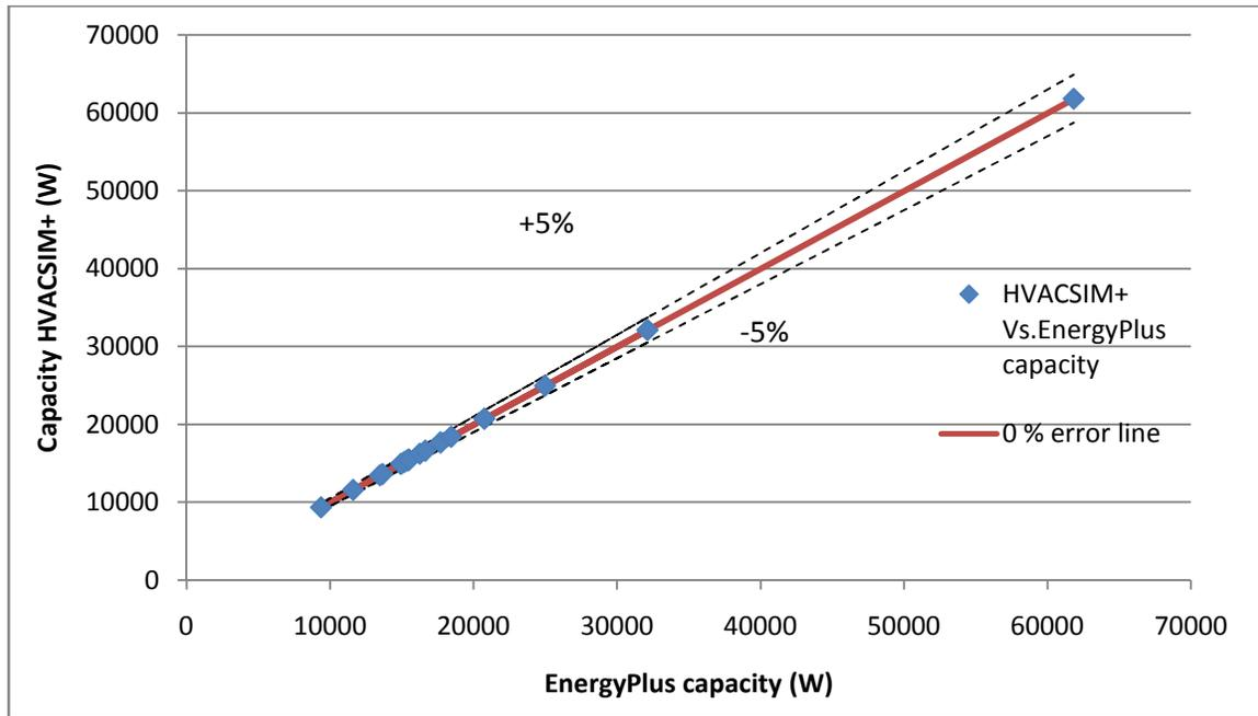
Fig. 5.2 EnergyPlus Vs HVACSIM+ capacity (W)
