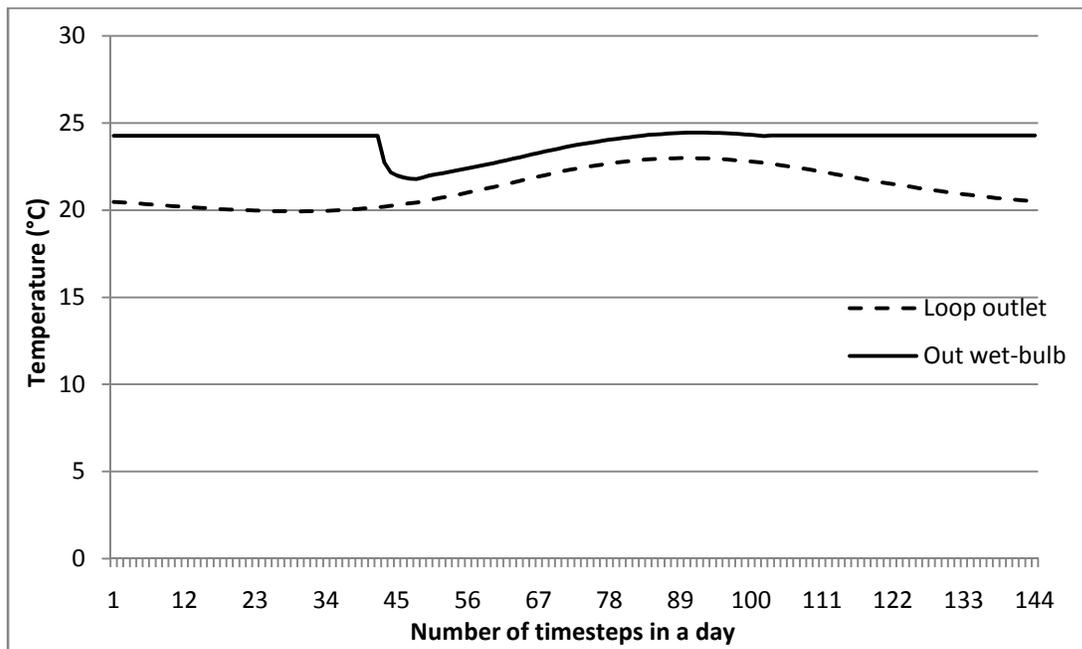
Fig 6.16 Air wet-bulb and loop outlet temperature on the design day
