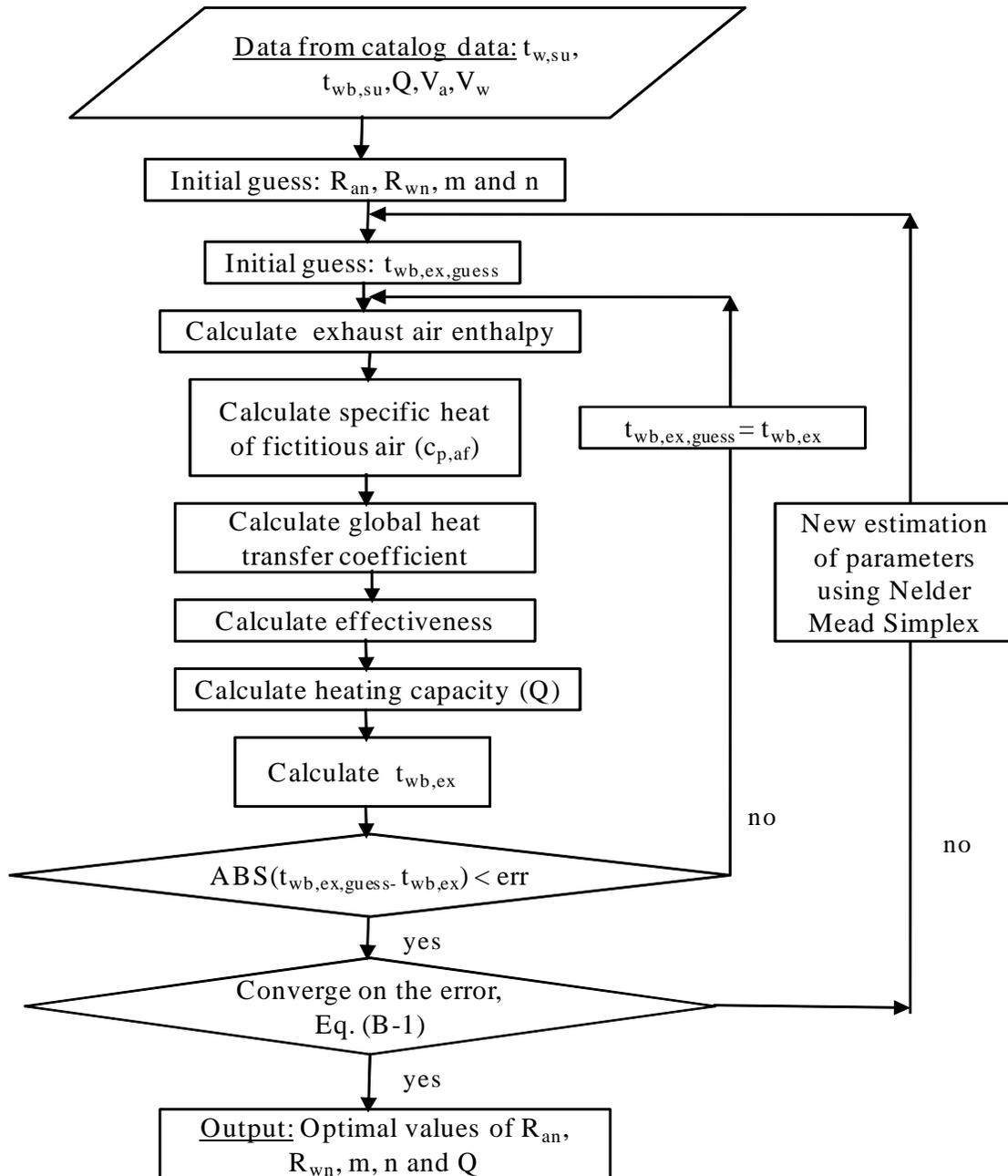
Fig B-1: Flow chart of Lebrun model implemented in VBA
