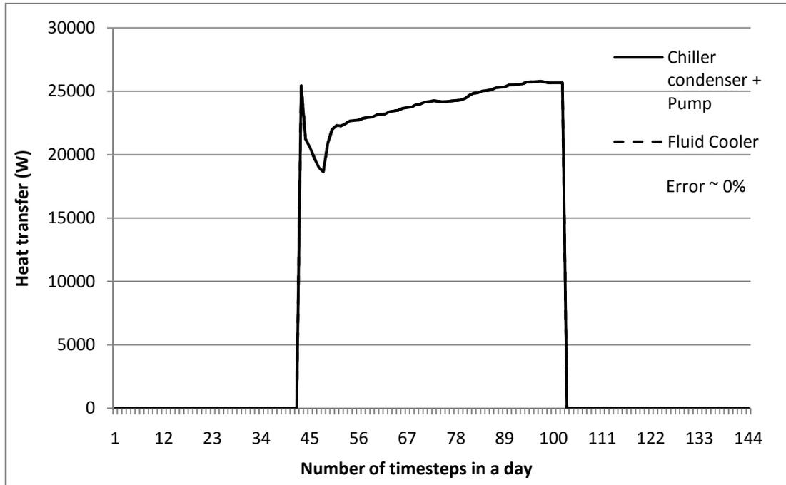
Fig 6.4 Condenser and pump heat addition vs. Fluid cooler heat transfer rate
