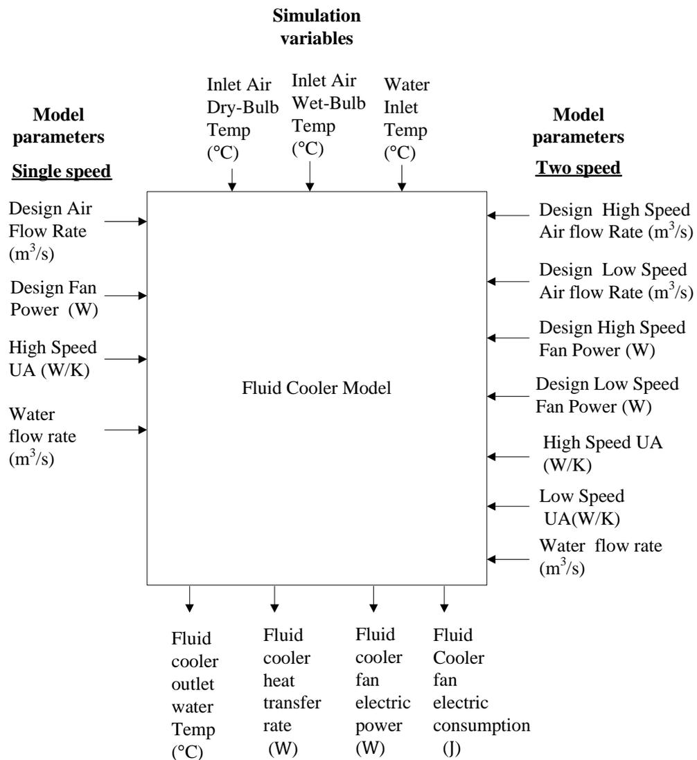
Fig 3.3: Information flow chart for UA and design flow rate method of fluid cooler model in EnergyPlus
