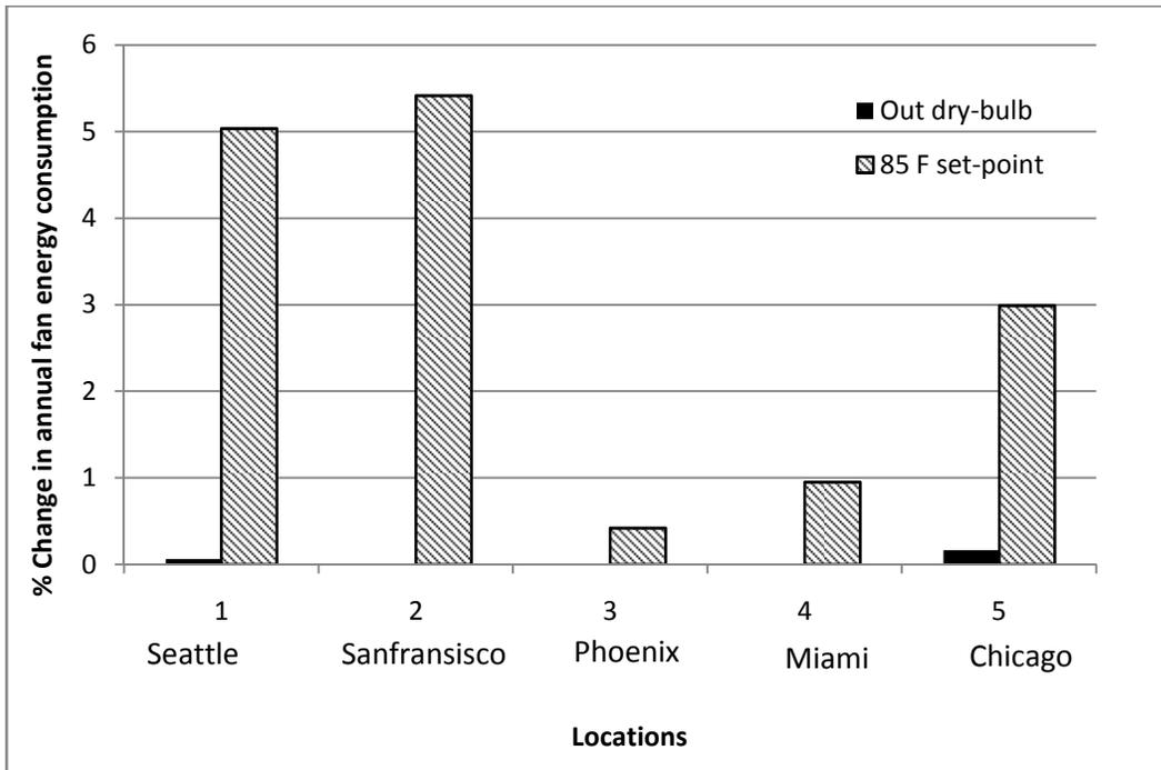
Fig 4.1 Comparison of % change in dry fluid cooler fan energy consumption due to change in UA value at different locations for two different set-points
