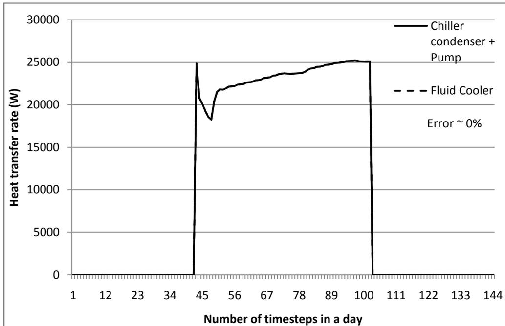
Fig 6.11 Condenser and pump heat addition vs. Fluid cooler heat transfer rate
