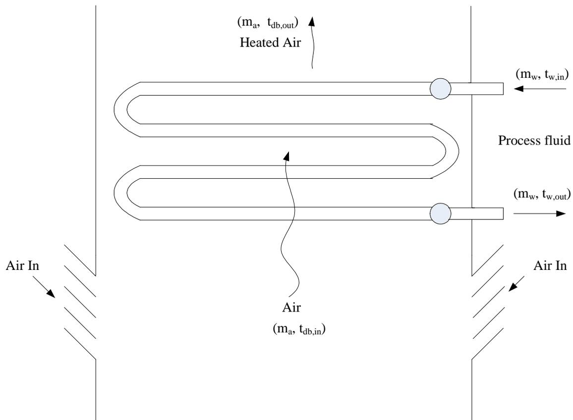
Fig 1.1 Schematic of dry fluid cooler
