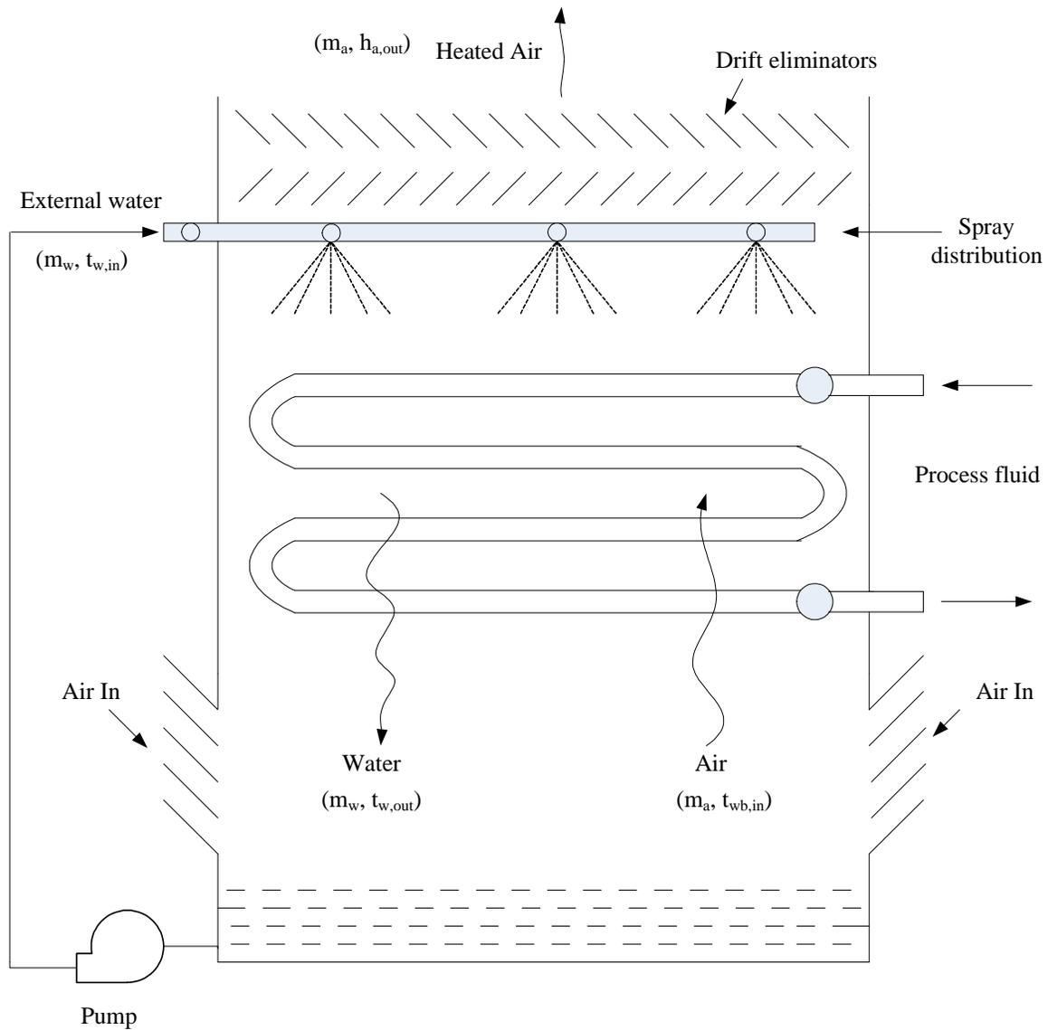
Fig 1.2 Schematic of evaporative fluid cooler
