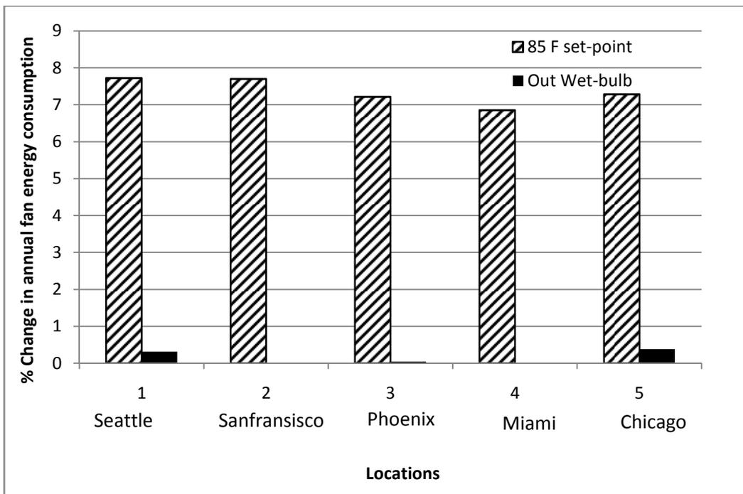
Fig 4.2 Comparison of % change in evaporative fluid cooler fan energy consumption due to change in UA value at different locations for two different set-points
