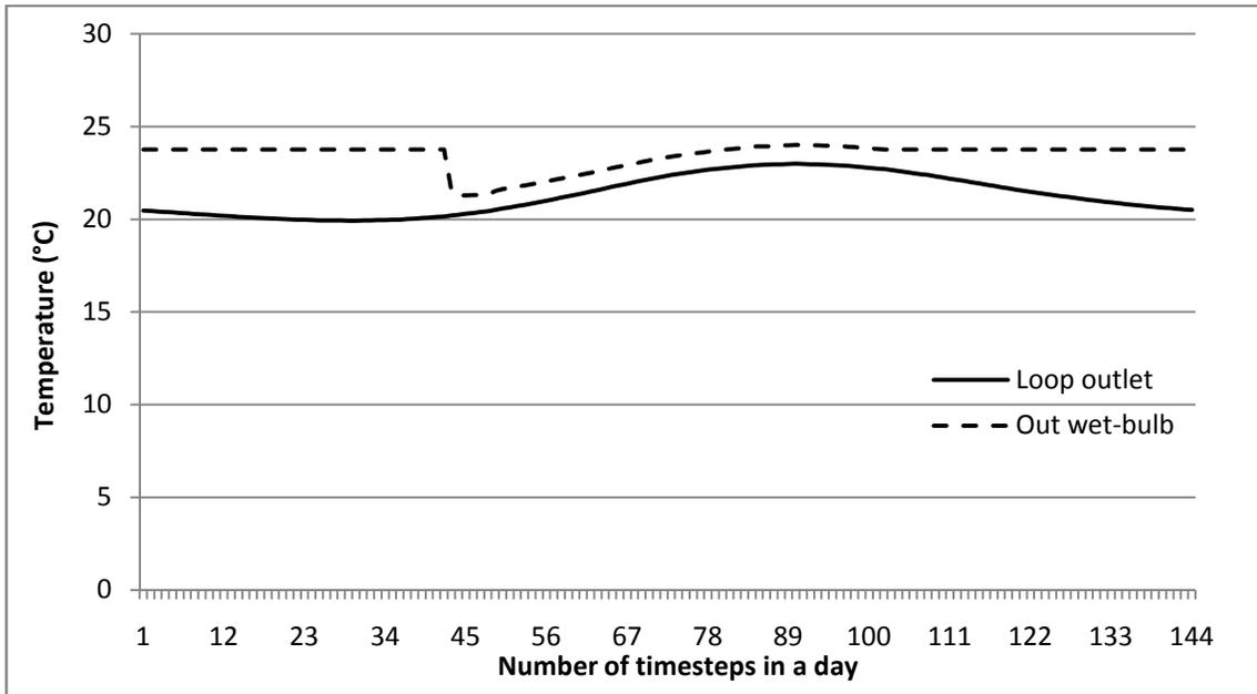
Fig 6.13 Air wet-bulb and loop outlet temperature on the design day
